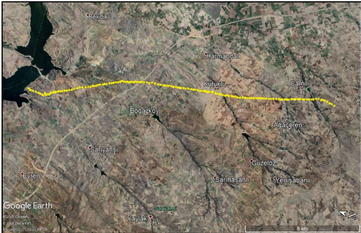
Figure 3 Planned Route of 34 kV ETL
